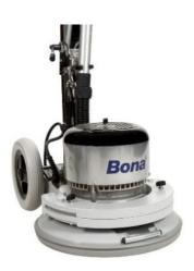
The Bona Power Drive<sup>®</sup> Weight Kit, comprised of two easy-to-mount 15 lb. weights, provides extra pressure to the Bona Power Drive<sup>®</sup>, making light work of tough sanding jobs as it allows you to customize the cutting power and sanding aggressiveness of the machine. One weight may even be used when wire-brushing for increased effect. (Note: Only one weight should be used when wire-brushing, as two may damage the brush heads.)
